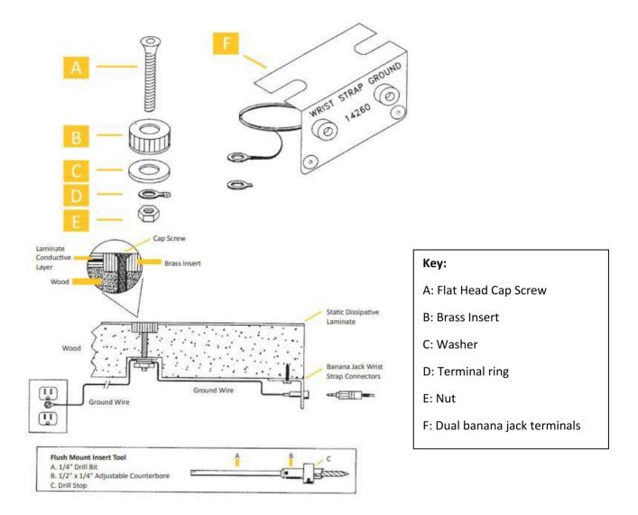
A high-quality lock-washer is used to give the screw a snug sit, preventing it from vibrating loose.
